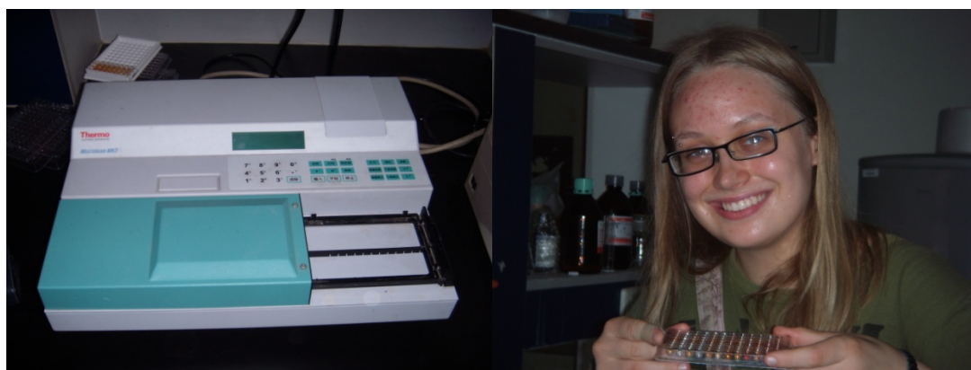
Figure 2: Absorbance Reader to left, me with completed ELISA test plate on right. Plates are inserted on the metal frame to the right of the light blue casing.
