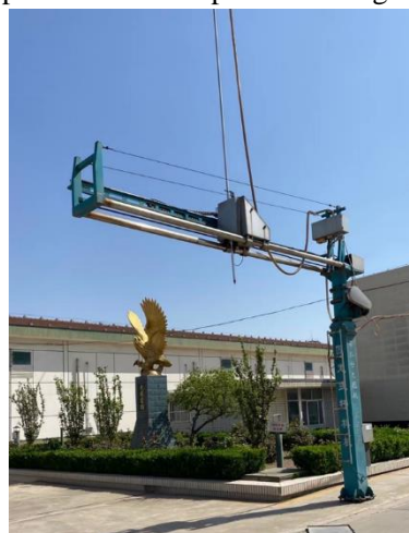
Figure 2 Prototype of the fixed sampler
