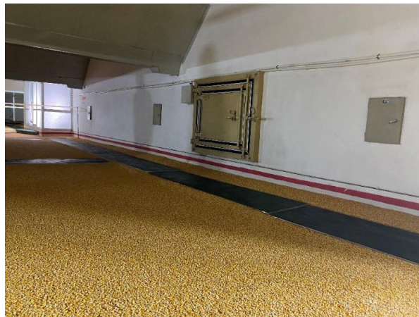
Figure 5 The height of grain surface decreased after the initial mechanical ventilation (Note: The initial height of grain surface of the granary is shown by the red line on the wall)
