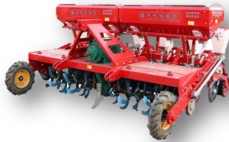
Figure 2. 2BMGF-6 Corn rotary tillage seeder
