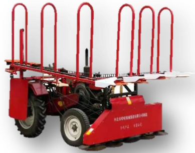
Figure 4. 4G-2.2CH corn stalk harvester
