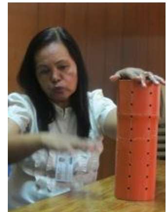
Figure 1: Engr. Evangeline Sibayan of PhilRice describes how to use a field water tube
