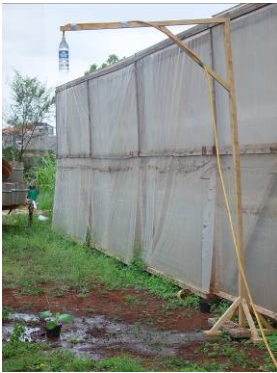
Figure 6: Rainfall simulator used a wooden frame that help plastic bottles that had holes drilled in the bottom to produce a varied levels of simulated rainfall.
