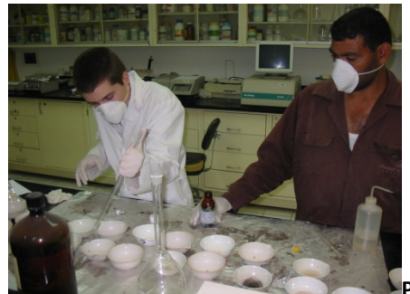
Preparing samples for analysis with the spectrometer to find nitrate absorbance
