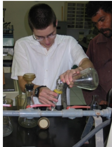
Using filtration to prepare water samples and analyze chlorophyll levels
