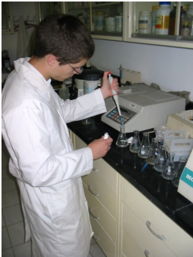
Analyzing phosphorous absorbance in order to determine the concentration
