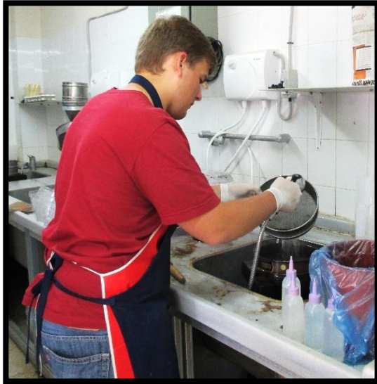
Picture 10: Each soil sample had to be washed and filtered through two sieves a total of three times. (Picture by Jiang Kuan Cui)
